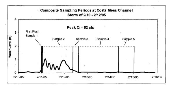
Flow-weighted compositing by field instrumentation (automatic sampler linked to portable flowmeter) has many disadvantages including:
