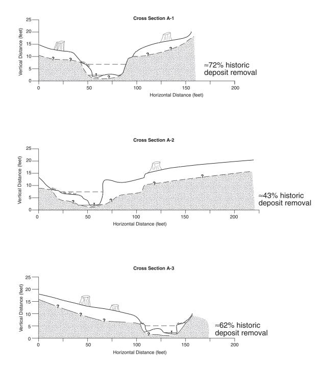
Figure 15. Surveyed cross sections A-1, A-2, and A-3. Dashed lines represent probable maximum thickness of historic aggradation used to estimate amount of material removed since time of terrace deposition.
