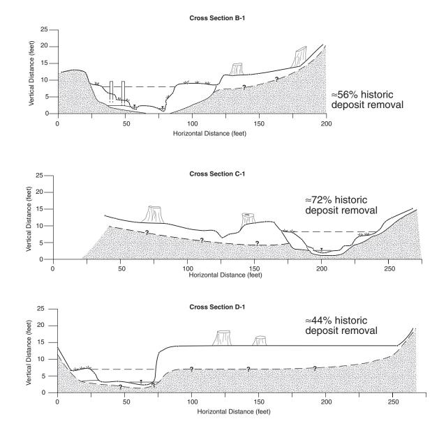
Figure 16. Surveyed cross sections B-1, C-1, and D-1. Dashed lines represent probable maximum thickness of historic aggradation used to estimate amount of material removed since time of terrace deposition.
