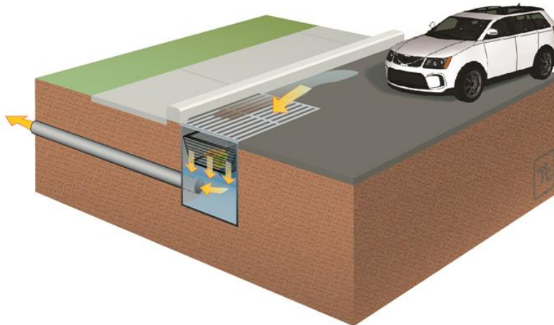
Figure 3-12: Pre-treatment BMP schematic
