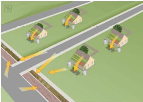
Figure 3-1: Distributed BMP Schematic
