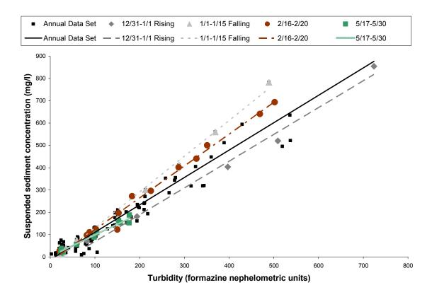
Figure 18. Suspended sediment concentration – turbidity relationship for annual data set and for selected storm events at Corrigan Creek.
