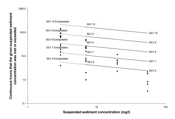
Figure 33. Continuous hours that a given suspended sediment concentration was met or exceeded at Little South Fork Elk River accompanied by Newcombe and Jensen model 4 severity of ill effects index (SEV) values for eggs and larvae of salmonids and non-salmonids.
