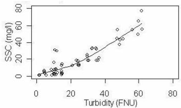
Figure 16. Low range of loess plot of suspended sediment concentration against turbidity for Little South Fork Elk River.
