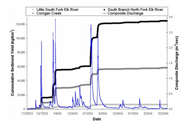
Figure 25. Sediment yield accumulation and composite discharge generated by averaging the discharges at Corrigan Creek, Little South Fork Elk River, and South Branch North Fork Elk River.
