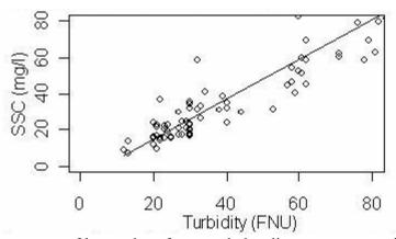
Figure 17. Low range of loess plot of suspended sediment concentration against turbidity for South Branch North Fork Elk River.
