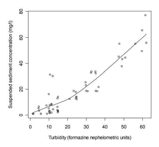
Figure 13. Loess plot of suspended sediment concentration against turbidity for Little South Fork Elk River.
