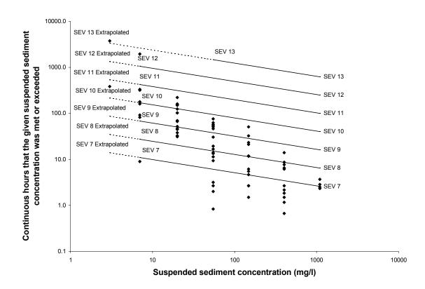
Figure 34. Continuous hours that a given suspended sediment concentration was met or exceeded at South Branch North Fork Elk River accompanied by Newcombe and Jensen model 4 severity of ill effects index (SEV) values for eggs and larvae of salmonids and non-salmonids.
