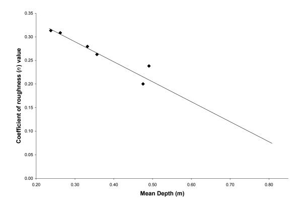
Figure 8. Computed coefficient of roughness (n) values against mean depth for discharge measurements at Little South Fork Elk River.
