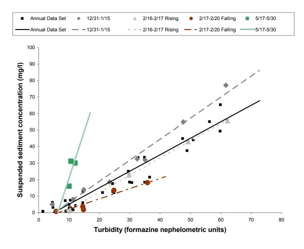
Figure 19. Suspended sediment concentration – turbidity relationship for annual data set and for selected storm events at Little South Fork Elk River.
