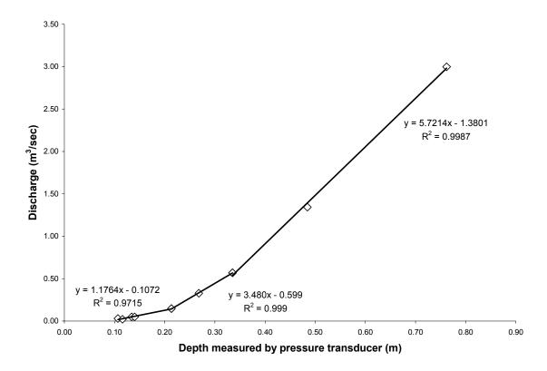
Figure 9. Three part linear discharge rating curve for Corrigan Creek.
