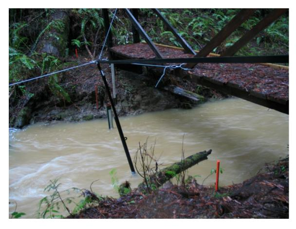
Figure 6. Bank mounted sampling boom articulating downstream during a high flow event on Corrigan Creek.
