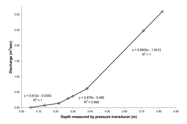
Figure 11. Three part linear discharge rating curve for South Branch North Fork Elk River.
