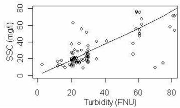
Figure 15. Low range of loess plot of suspended sediment concentration against turbidity for Corrigan Creek.
