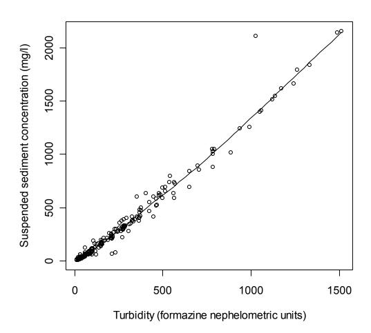
Figure 14. Loess plot of suspended sediment concentration against turbidity for South Branch North Fork Elk River.
