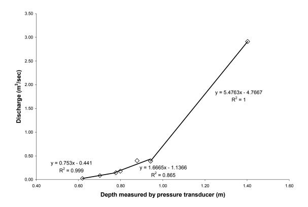
Figure 10. Three part linear discharge rating curve for Little South Fork Elk River.
