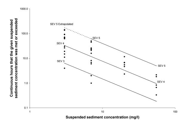
Figure 30. Continuous hours that a given suspended sediment concentration was met or exceeded at Little South Fork Elk River accompanied by Newcombe and Jensen model 1 severity of ill effects index (SEV) values for juvenile and adult salmonids.
