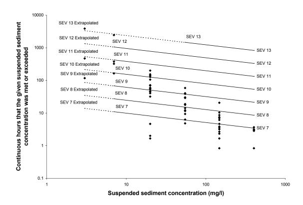
Figure 32. Continuous hours that a given suspended sediment concentration was met or exceeded at Corrigan Creek accompanied by Newcombe and Jensen model 4 severity of ill effects index (SEV) values for eggs and larvae of salmonids and non-salmonids.
