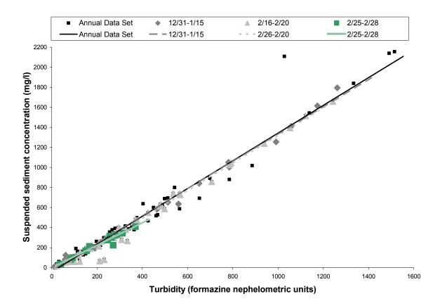
Figure 20. Suspended sediment concentration – turbidity relationship for annual data set and for selected storm events at South Brach North Fork Elk River.
