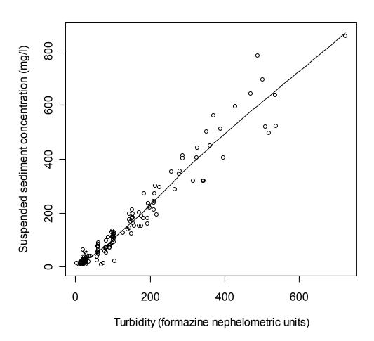
Figure 12. Loess plot of suspended sediment concentration against turbidity for Corrigan Creek.
