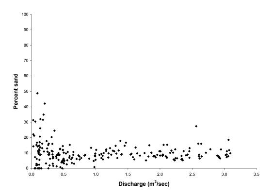
Figure 23. Percent sands as a function of discharge at South Branch North Fork Elk River.
