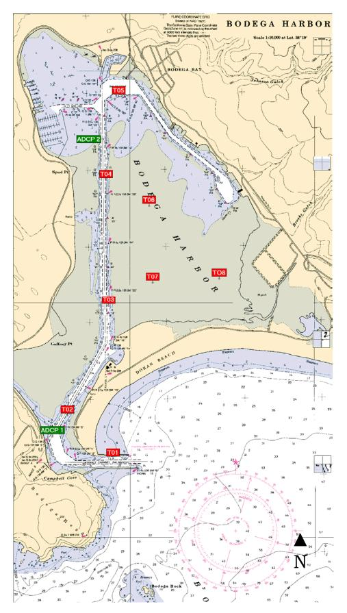
**Figure 2.** Bodega Harbor. Moored instrument positions are shown for current profilers (ADCP's, green) and temperature sensors (red).
