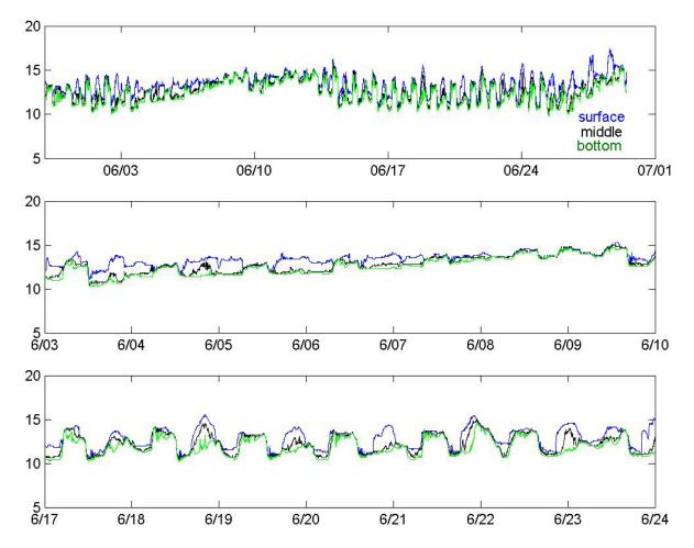
Figure 58. Temperature at rear harbor mooring (Porto Bodega), Spring 2003. Top: full record. Center: week of June 3-10. Bottom: week of June 17-24.
