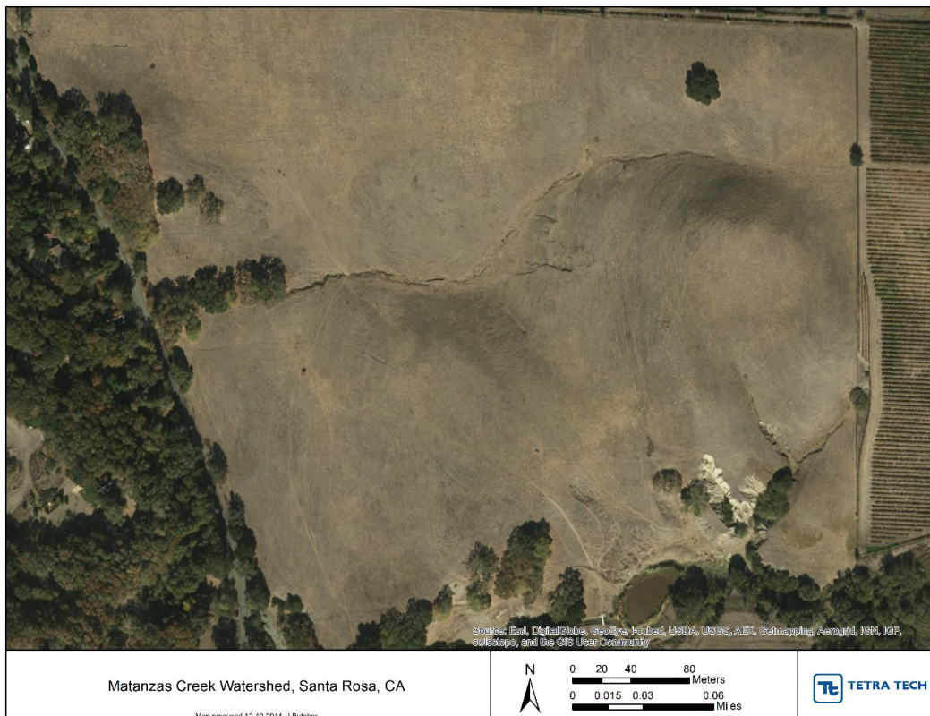
Figure 6-1. Example of Enlarging Gullies upstream of Matanzas Reservoir
