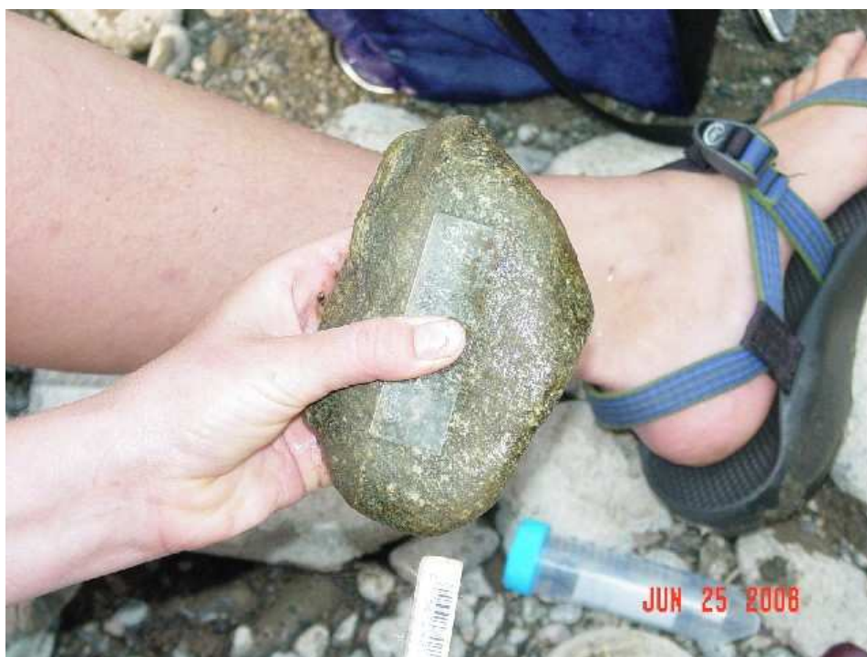
Figure 6.6.2 Sample area equivalent to a 1" X 3" microscope slide is selected prior to scraping. Photo was taken by KTWQP staff at Klamath River Orleans site in June 2006.
