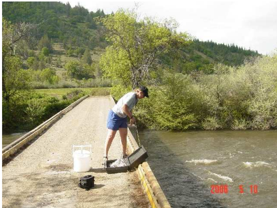
Figure 6.5.1. KTWQP staff collects Klamath River water using a Van dorn sampler and then deposits in churn to ensure representativeness of sample. Photo taken in 2006 at Klamath River above Copco Reservoir.
