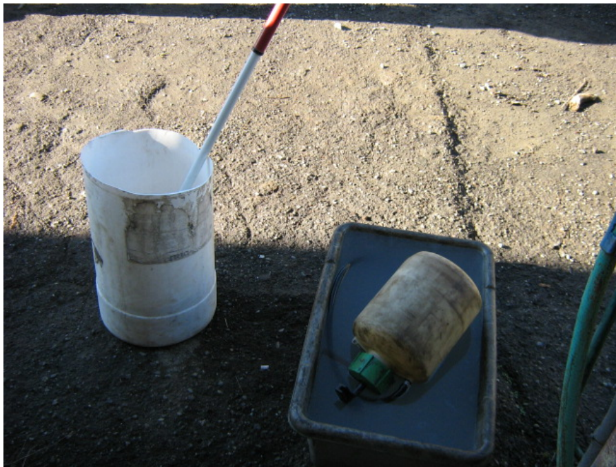
Photograph 20: Wash equipment used in the absence of structural vehicle and equipment washing BMPs at the Healdsburg Corporate Yard
