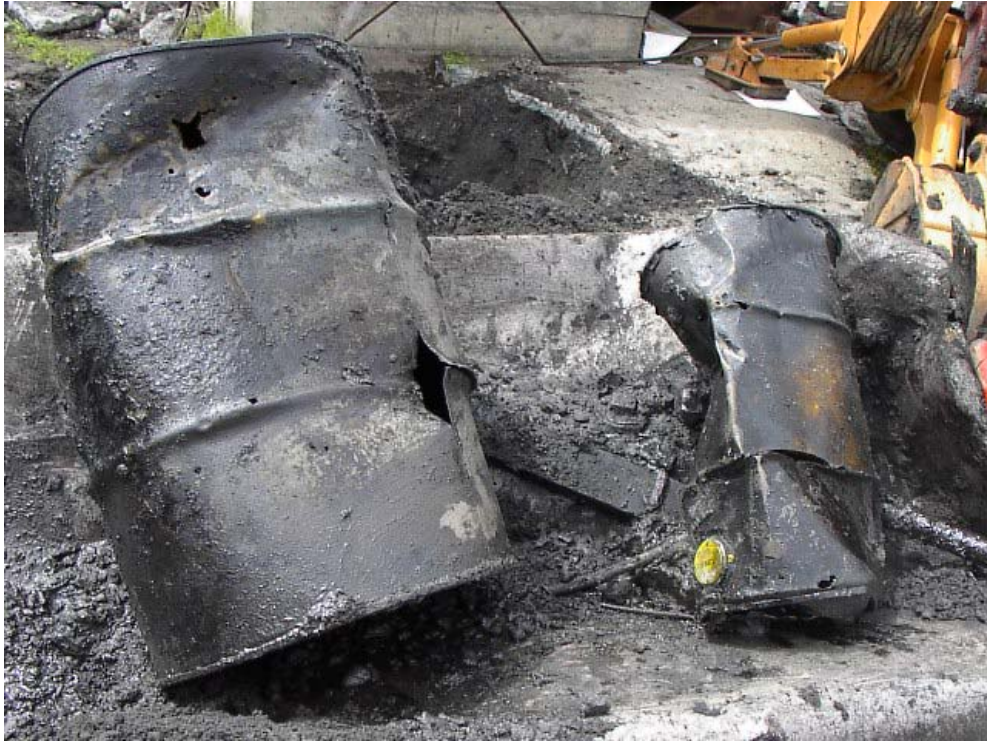
55 gallon and 30 gallon drums removed during tank removal.
