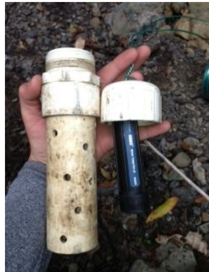
Figure 6. Stream temperature logger with protective PVC case.
