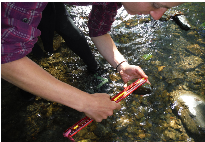
Figure 2. Measuring particle size (mm) of the streambed surface.
