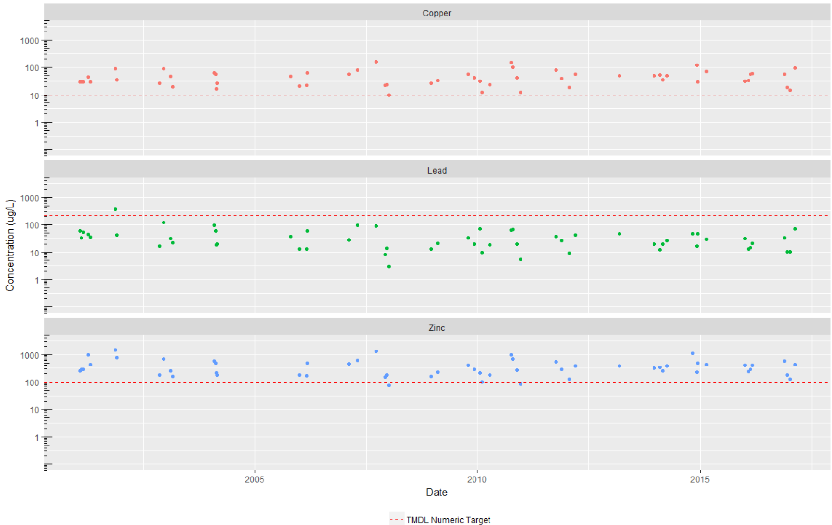
Total Metals Measured During Wet Weather Events - Los Cerritos Channel @ Stearns Street (2000 to 2017)
