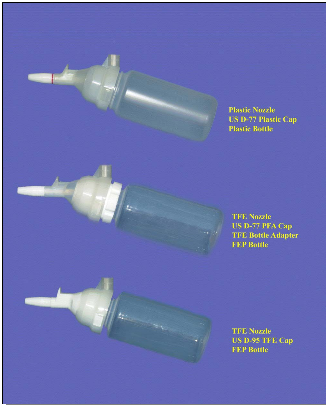
Figure 2. US DH-81 sampler cap/bottle combinations
