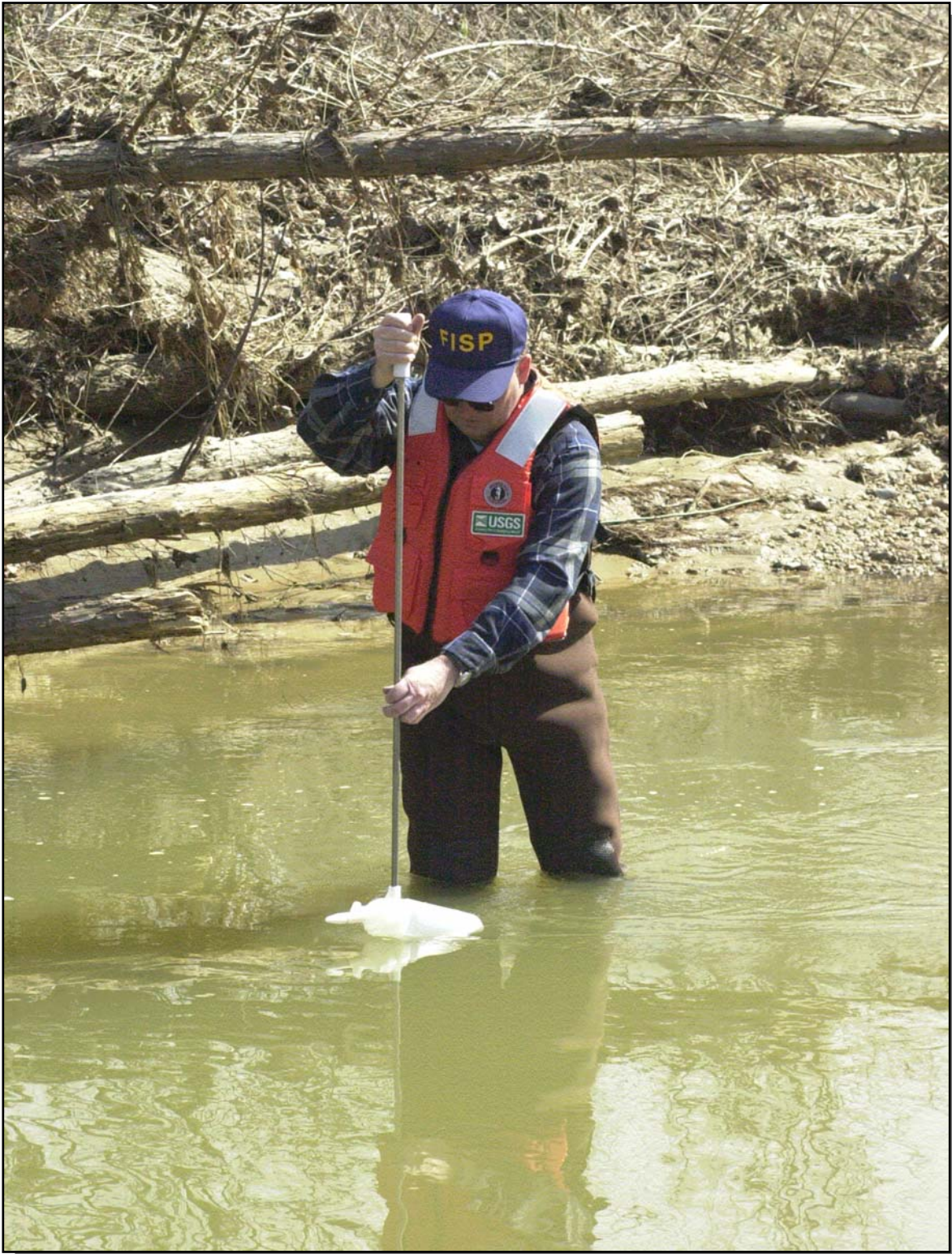
Figure 15. Example of proper position for sampling
