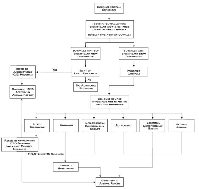
Figure 5-1 Non-Stormwater Outfall Program Flow Diagram
