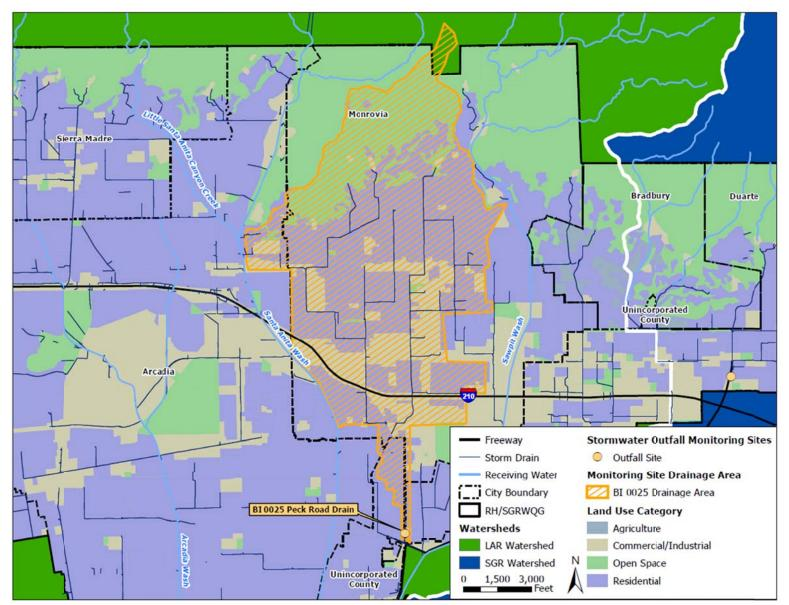
Figure 4-5 Stormwater Outfall Monitoring Site – City of Monrovia
