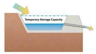
Figure 3-4 Conceptual Diagram Illustrating Storage
