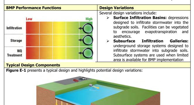
Figure E-1 Typical Regional Infiltration Facility Schematic (arrows indicate water pathways)
