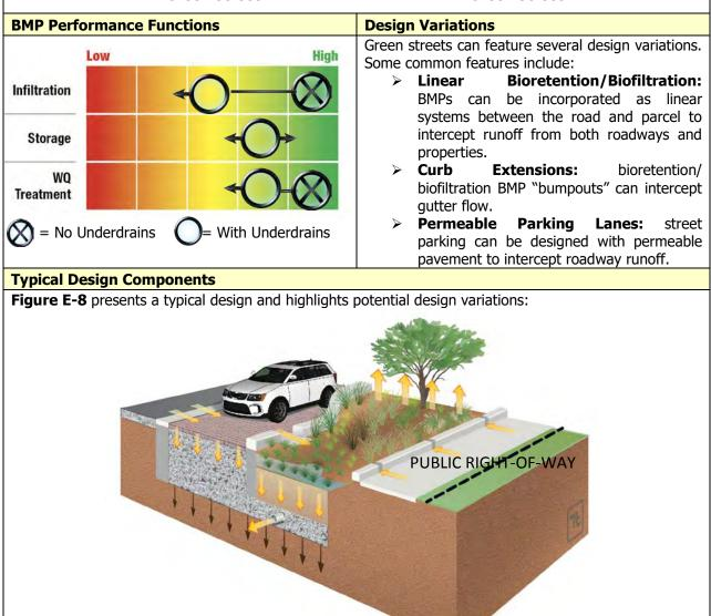
Figure E-8 Typical Distributed Green Street Schematic (arrows indicate water pathways)
