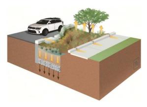
Figure 3-4: Bioretention without underdrain schematic
