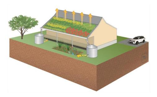
Figure 3-13: Above ground cisterns schematic
