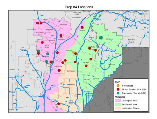
Figure 3-17: BMP Locations within the Gateway Prop 84 Project
