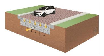
Figure 3-6: Porous pavement schematic
