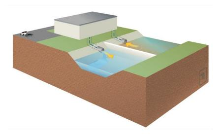
Figure 3-15: Low flow diversion schematic
