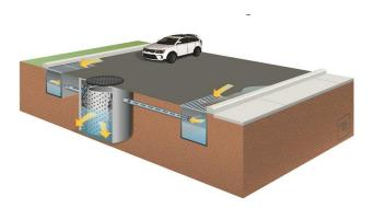
Figure 3-5: Drywell schematic
