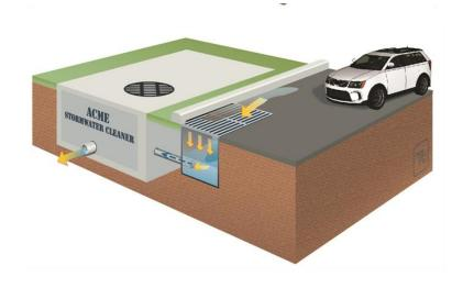
Figure 3-14: Underground detention schematic
