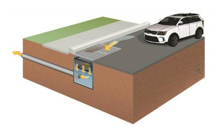
Figure 3-12: Pre-treatment BMP schematic
