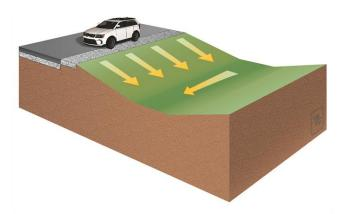
Figure 3-9: Vegetated swale schematic
