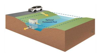
Figure 3-10: Wet detention basin schematic
