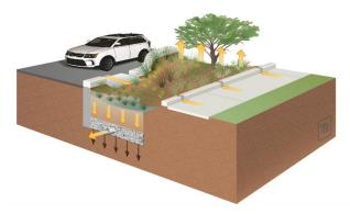
Figure 3-8: Bioretention with Underdrains schematic
