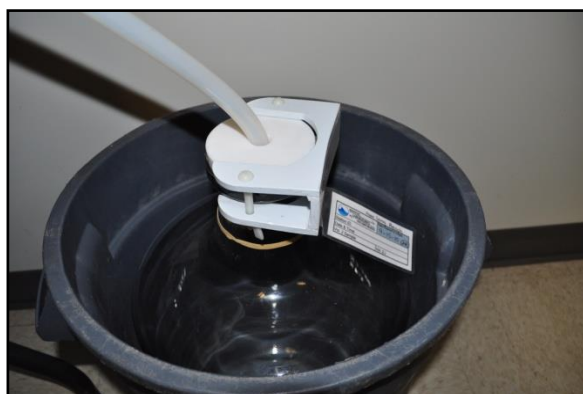
Figure 1. Composite Bottle with Label and installed Tubing inside Brute® Container.
