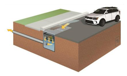
Figure 3-12: Pre-treatment BMP schematic
