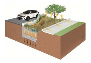
Figure 3-4: Bioretention without underdrain schematic
