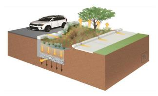
Figure 3-8: Bioretention with Underdrains schematic
