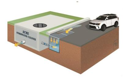
Figure 3-14: Underground detention schematic
