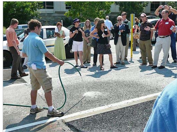
Demonstrating water infiltration through pervious concrete (left) and porous asphalt (right). Parking lot at Villanova University, Pennsylvania. EPA / Abby Hall
