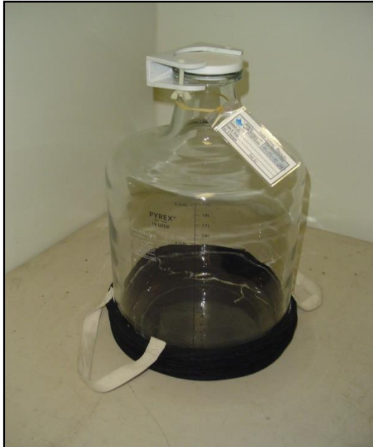
Figure 2. Composite bottle showing bottle bag used for transport and lifting.
