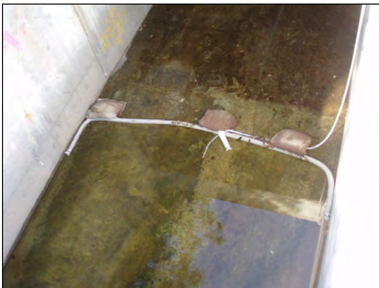
Figure 9-8. Typical Wet-Season, Dry-Weather Sampling Configuration
