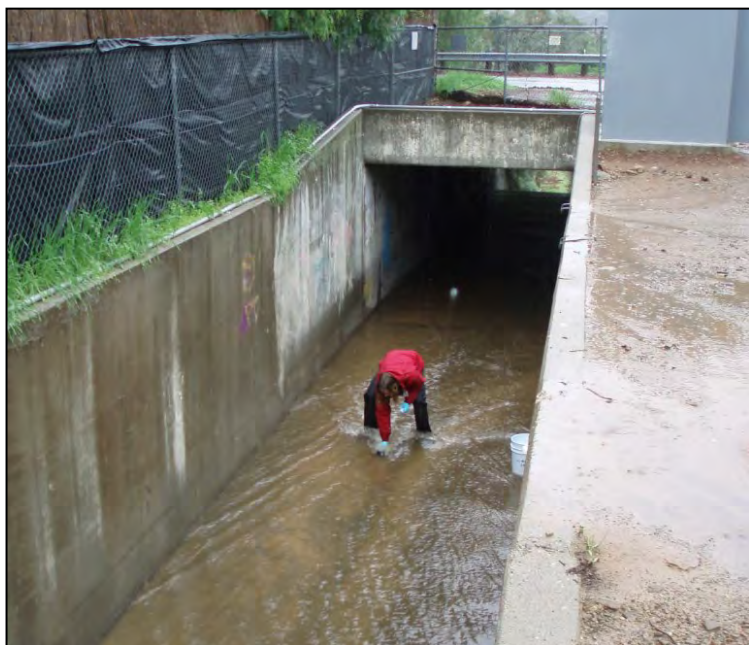
Figure 9-9-6. Grab Sampling at Mid-Stream, Mid-Depth
