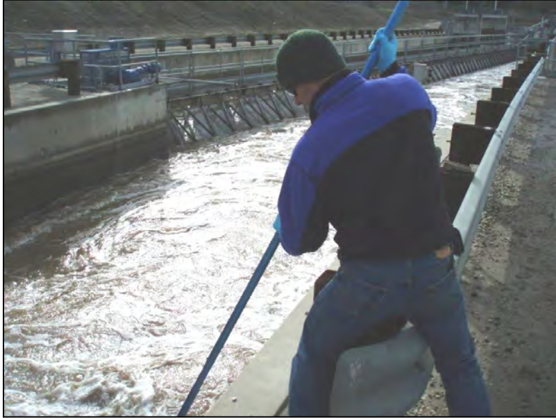
Figure 9-7. Grab Sampling Using Extended-Reach Swing Sampler
