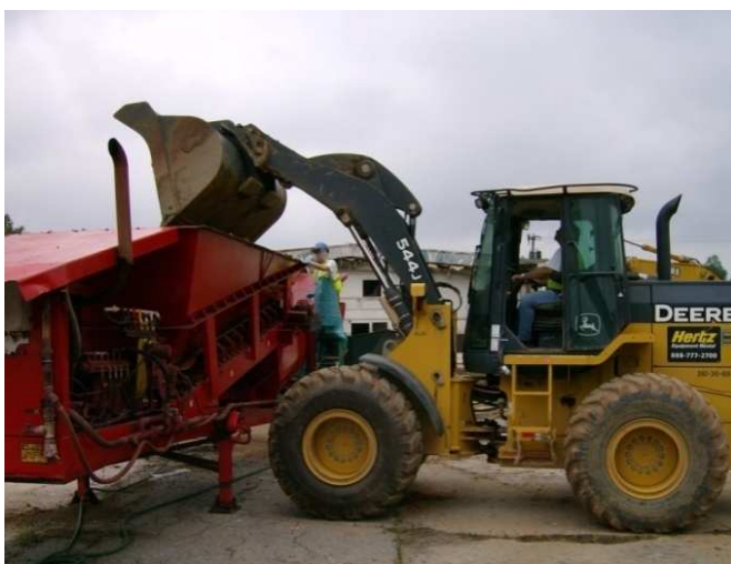
Figure 2: Transfer of soil into cells for treatment with VeruSOLVE™.
