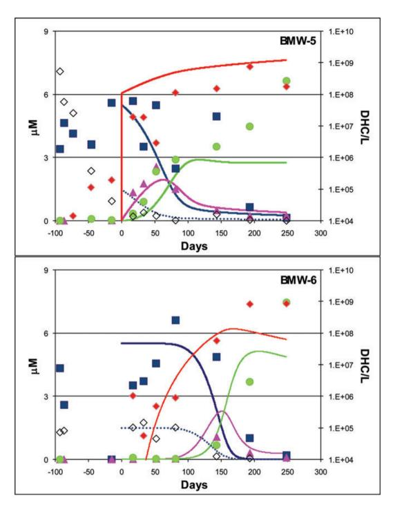
Figure 5. Ethenes and DHC concentrations plotted as a function of time for loop 3. Bioaugmentation was performed at 0 days.  $\Diamond$ , TCE;  $\blacksquare$ , DCE;  $\triangle$ , vinyl chloride;  $\bigcirc$ , ethene;  $\bigcirc$ , DHC. Solid and dotted lines represent corresponding model simulations. Simulated DHC concentrations in the bioaugmentation injection well (BMW-5) include the total (mobile and immobile) DHC.
