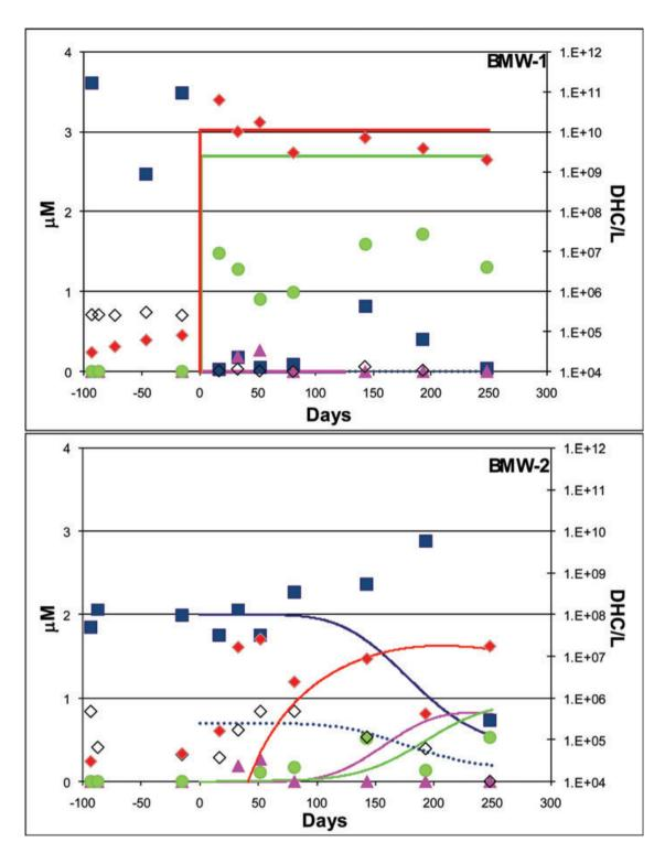
Figure 3. Ethenes and DHC concentrations plotted as a function of time for loop 1. Bioaugmentation was performed at 0 days.  $\Diamond$ , TCE;  $\blacksquare$ , DCE;  $\triangle$ , vinyl chloride;  $\bigcirc$ , ethene;  $\bigcirc$ , DHC. Solid and dotted lines represent corresponding model simulations. Simulated DHC concentrations in the bioaugmentation injection well (BMW-1) include the total (mobile and immobile) DHC.
