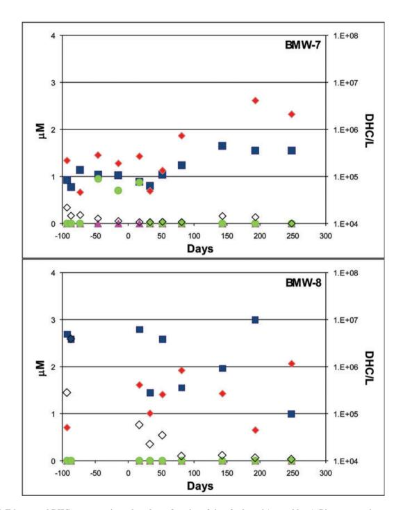
Figure 6. Ethenes and DHC concentrations plotted as a function of time for loop 4 (control loop). Bioaugmentation was performed at 0 days.  $\Diamond$ , TCE;  $\blacksquare$ , DCE;  $\triangle$ , vinyl chloride;  $\bigcirc$ , ethene;  $\bigcirc$ , DHC. No detection of vinyl chloride or ethene were observed.
