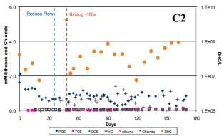
FIGURE 3. Effluent concentrations of ethenes, chloride, and DHC from rock C1 (top) and C2 (bottom) in Experiments 5 and 6, respectively. Fractures were bioaugmented on Day 0. The vertical lines indicate when the fractures flow was decreased or when inoculation with additional culture was performed.
