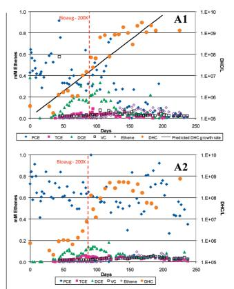
FIGURE 1. Effluent concentrations of ethenes and DHC from rock A1 (top) and A2 (bottom) in Experiments 1 and 2, respectively. Fractures were bioaugmented on Day 0. The vertical dashed lines indicate when inoculation with additional culture was performed. The solid line for A1 represents the predicted rate of DHC growth (5). For A2, some interruptions in flow occurred between days 150 and 190. Chloride concentrations were not monitored in Experiments 1 and 2.
