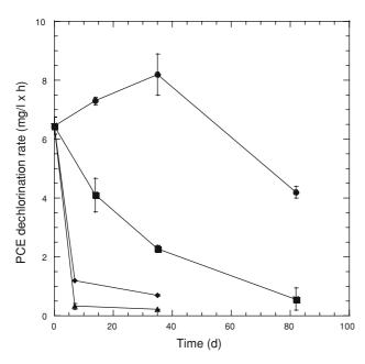
**Fig. 5** Effect of storage conditions on the activity of concentrated SDC-9<sup>TM</sup> culture. Tenfold-concentrated SDC-9<sup>TM</sup> culture was stored anaerobically and without substrate at either 4°C (filled circle), 13°C (filled square), 22°C (filled diamond) or 28°C (filled triangle). Values represent means of triplicate samples, and *error bars* are one standard error of the mean
