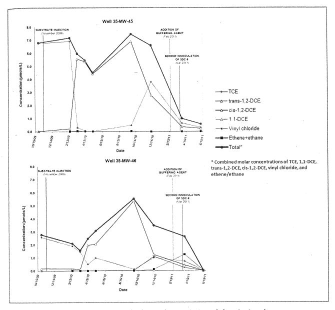
**Exhibit 5.** Molar concentrations of VOCs at the downgradient monitoring wells from the time of the biobarrier installation until June 2011
