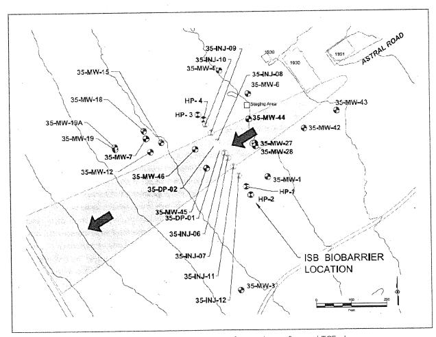
**Exhibit 1.** The arrows indicate the approximate direction of groundwater flow and TCE plume migration. The plume contour represents the approximate 50 micrograms per liter TCE in groundwater prior to the biobarrier installation
