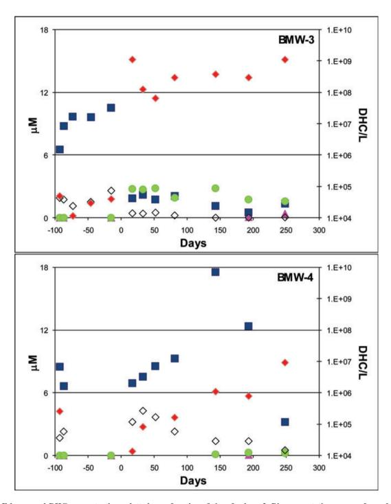
Figure 4. Ethenes and DHC concentrations plotted as a function of time for loop 2. Bioaugmentation was performed at 0 days.  $\Diamond$ , TCE;  $\blacksquare$ , DCE;  $\triangle$ , vinyl chloride;  $\bigoplus$ , ethene;  $\bigoplus$ , DHC.
