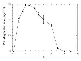
**Fig. 3** Effect of culture pH on PCE dehalogenation by SDC-9<sup>TM</sup>. Values represent the mean of triplicate samples, and *error bars* represent one standard error of the mean
