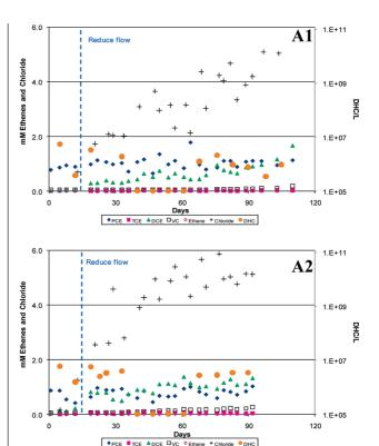
FIGURE 2. Effluent concentrations of ethenes, chloride, and DHC from rock A1 (top) and A2 (bottom) in Experiments 3 and 4, respectively. Fractures were bioaugmented on Day 0. The vertical lines indicate when the fractures flow was decreased from approximately 0.10 cm³/min to 0.025 cm³/min. Experiment 4 was terminated prior to Experiment 3.
