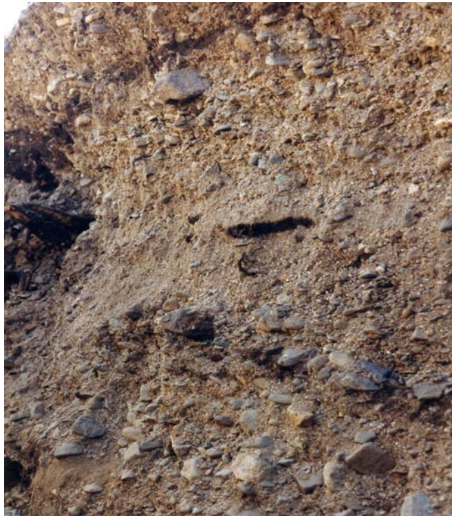
Figure 3. Photographs showing coarse-grained gravel and sand of proximal alluvial fan deposits beneath the main parking lot at Squaw Valley. (Photos courtesy of B. Hecht)
