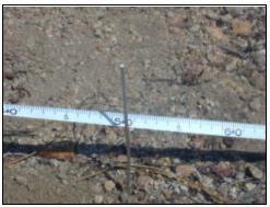
Figure 44. Erosion pin for measuring rates of sediment movement on hillslopes.
