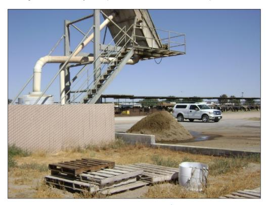
Figure 4.1: This machine, as a BMP, is used for separating manure solids from liquids. The liquids will be reused and applied as crop irrigation and fertilization water, increasing removal of nitrogen through crop uptake and decreasing nitrogen available for transport to groundwater.
