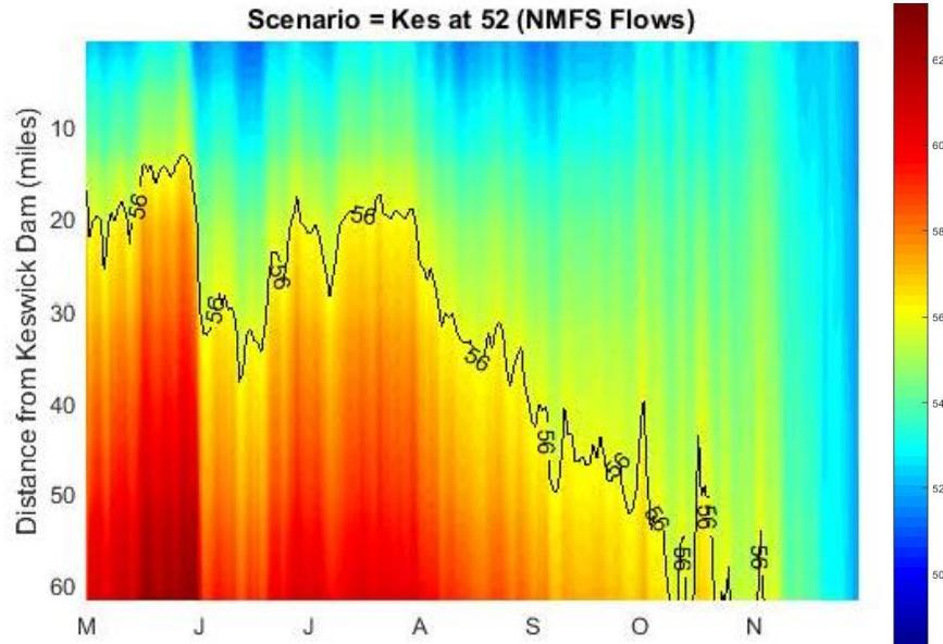
**Figure 8. NMFS-SWFSC RAFT model results using the 2016 February 90% exceedance outlook, historical 10% local 3-month temperature outlook meteorology, NMFS scenario for Keswick Dam monthly average releases for May through November, and targeting approximately 52°F DAT at KWK.**
