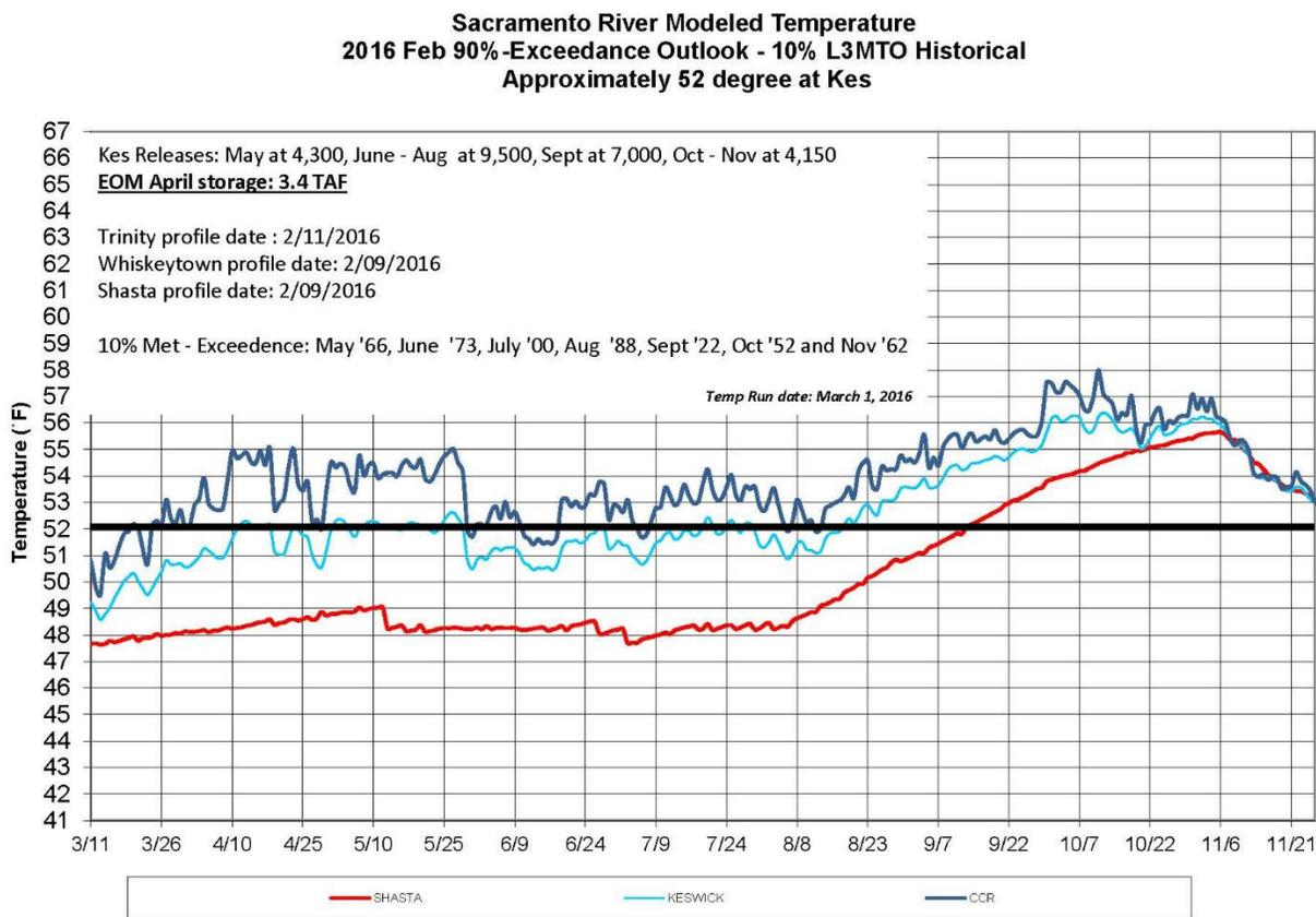
**Figure 4. Reclamation’s Sacramento River Modeled Temperature Results using the 2016 February 90% exceedance outlook, historical 10% local 3-month temperature outlook meteorology, Reclamation’s proposed Keswick Dam monthly average releases for May through November, and targeting approximately 52°F DAT at KWK.**
