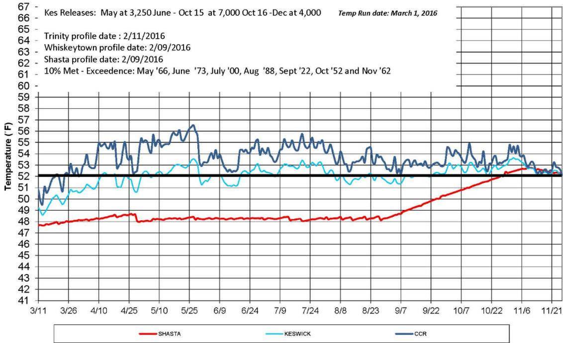
**Figure 7. Reclamation’s Sacramento River Modeled Temperature Results using the 2016 February 90% exceedance outlook, historical 10% local 3-month temperature outlook meteorology, NMFS-scenario for Keswick Dam monthly average releases for May through November, and targeting approximately 52°F DAT at KWK.**
