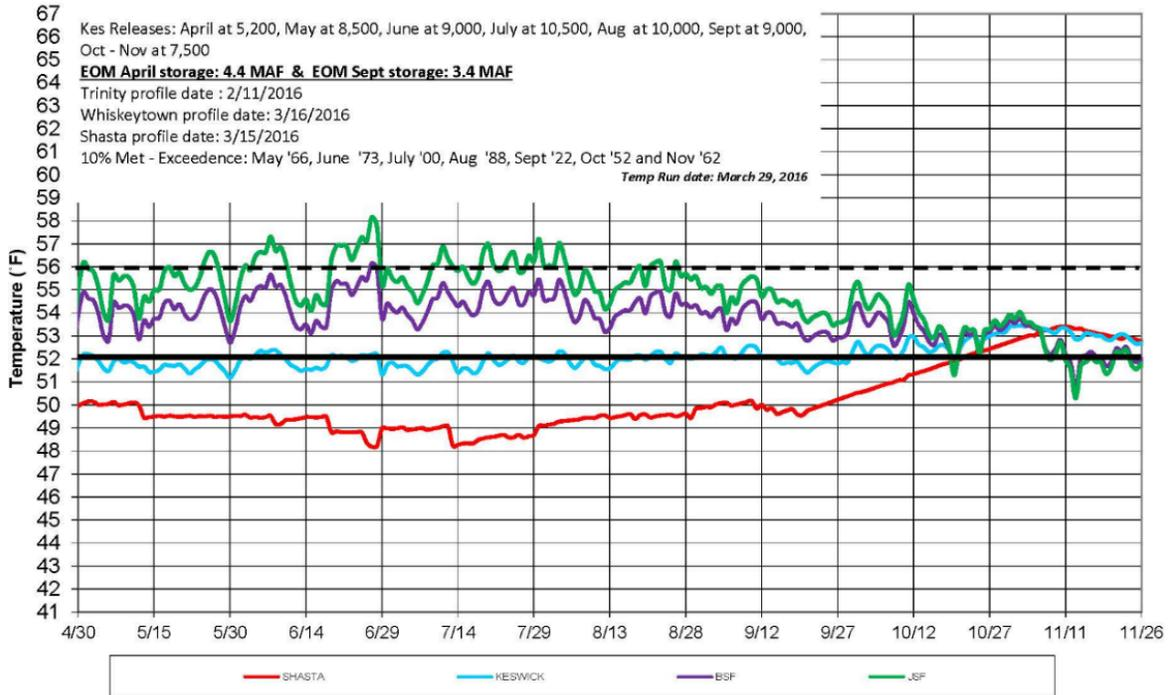
**Figure 2. SRWQM Results for May through November using the 2016 March 50% exceedance outlook, historical 10% local 3-month temperature outlook meteorology, Reclamation’s proposed Keswick Dam monthly average releases, and targeting approximately 52°F DAT at KWK.**
