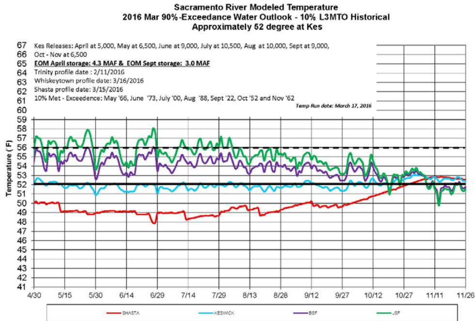
**Figure 1. Reclamation’s Sacramento River Water Quality Model (SRWQM) Temperature Results for May through November using the 2016 March 90% exceedance outlook, historical 10% local 3-month temperature outlook meteorology, Reclamation’s proposed Keswick Dam monthly average releases, and targeting approximately 52°F DAT at KWK.**
