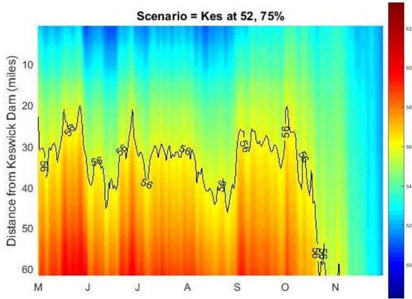
**Figure 10. NMFS-SWFSC RAFT model results using the 2016 February 75% exceedance outlook, historical 10% local 3-month temperature outlook meteorology, Reclamation’s proposed Keswick Dam monthly average releases for May through November, and targeting approximately 52°F DAT at KWK.**
