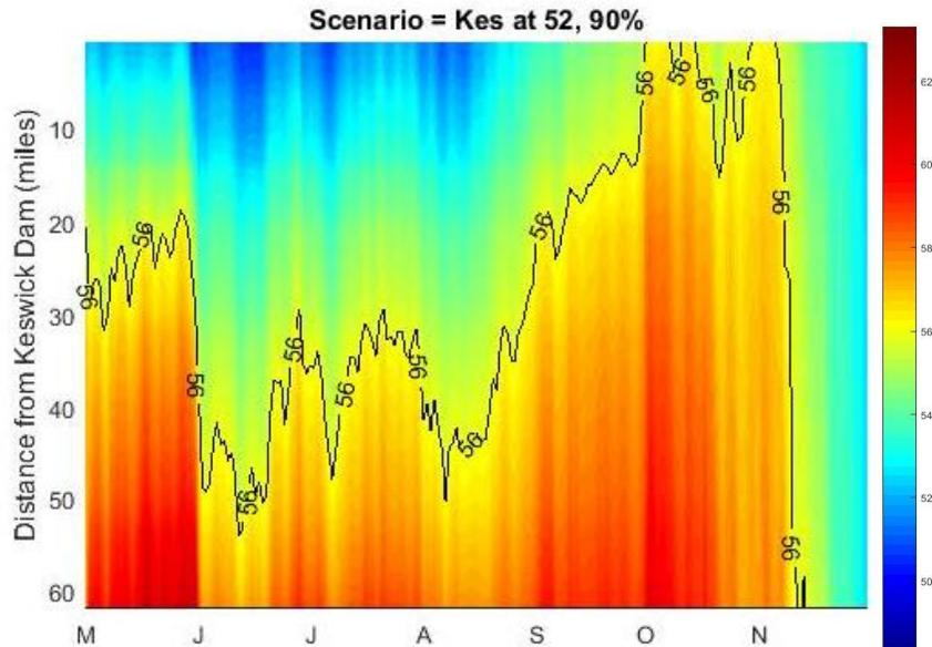
**Figure 5. NMFS-SWFSC RAFT model results using the 2016 February 90% exceedance outlook, historical 10% local 3-month temperature outlook meteorology, Reclamation’s proposed Keswick Dam monthly average releases for May through November, and targeting approximately 52°F DAT at KWK.**
