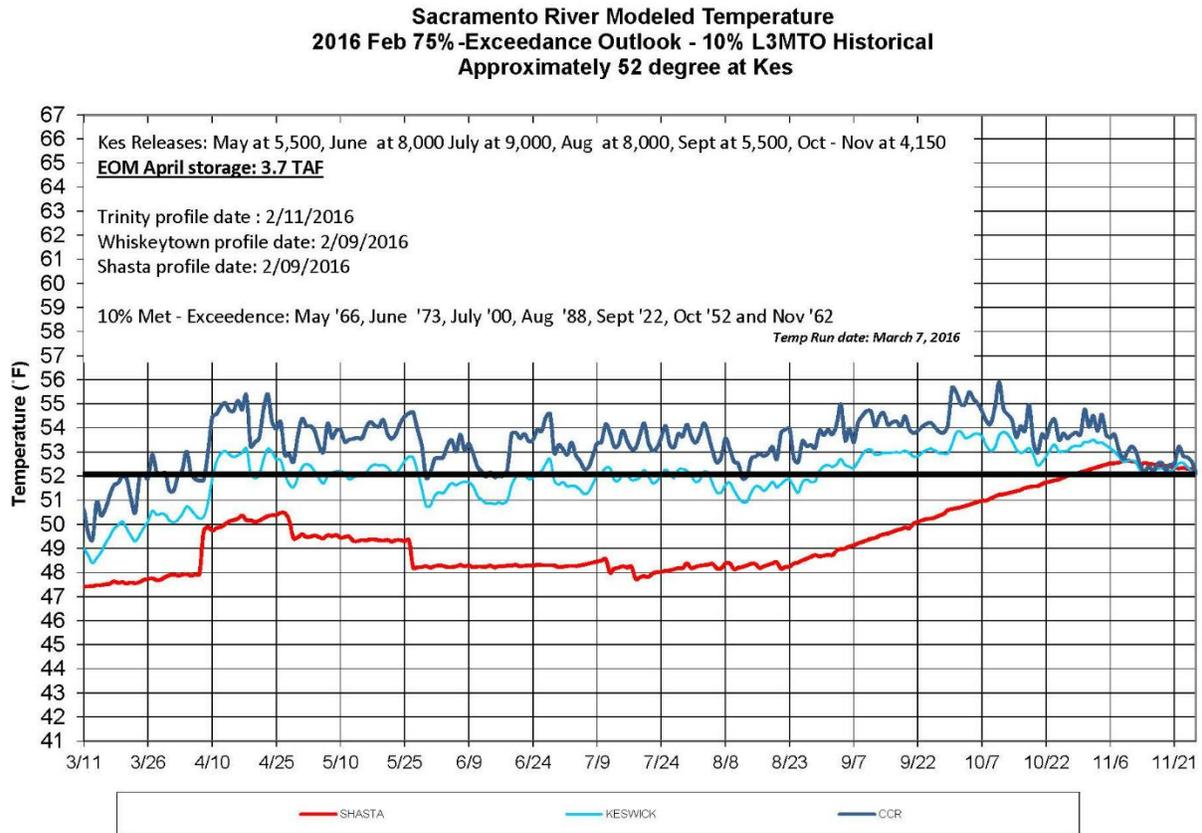
**Figure 9. Reclamation’s Sacramento River Modeled Temperature Results using the 2016 February 75% exceedance outlook, historical 10% local 3-month temperature outlook meteorology, Reclamation’s proposed Keswick Dam monthly average releases for May through November, and targeting approximately 52°F DAT at KWK.**
