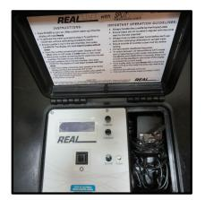
**Source %UVT/UVA.** Source water %UVT/UVA was measured to provide a comparison to filtrate water. Suspended solids can interfere with %UVT/UVA measurements regarding the absorption of indirect dissolved organic carbon. For true %UVT/UVA measurements, source water samples should be filtered directly into a cuvette using a 0.4 µm absolute size Isopore membrane to remove most suspended solids applying the same filterability technique for filtrate water analysis.
