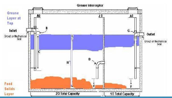
Main components: Inlet T, Midwall Baffle, Outlet T
