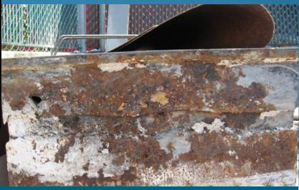
Floor trap that has rusted. Many traps that have been installed in floors were never designed for below floor installation
