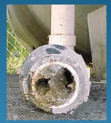
Outlet pipe of trap with no flow restrictor
