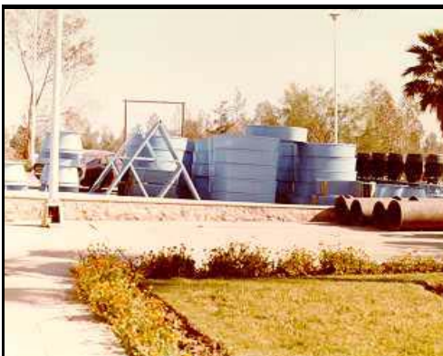
Figure 48: Aerator units for Mexicali's sewage lagoons. Although installed, the units did not function (Mar 1982)
