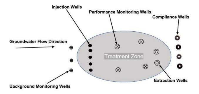
Figure 1: Generalized Monitoring Well Network Diagram
