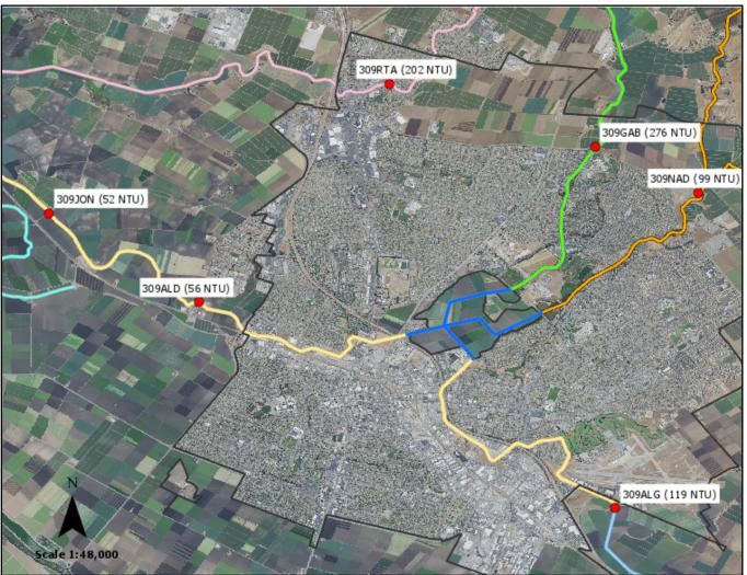
Figure 17. Map of water quality monitoring sites around the City of Salinas and median turbidity levels in parenthesis.
