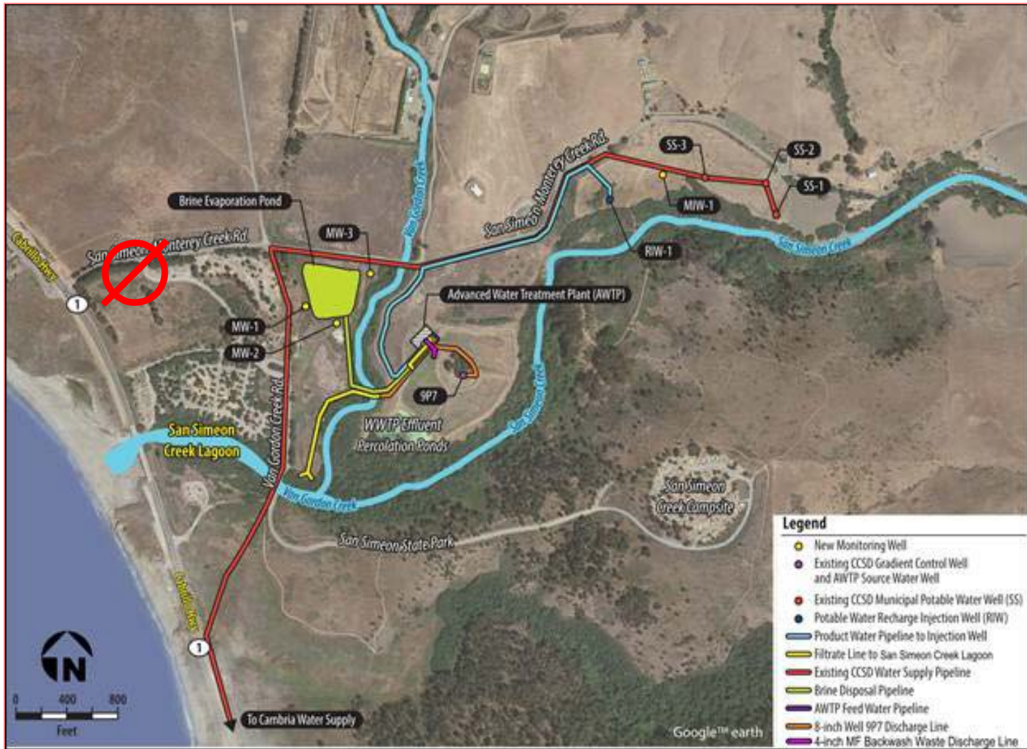
Figure 2 - Emergency Water Supply Project (Extraction Well, Treatment Plant, Percolation Ponds, Groundwater Injection Site, Water Supply Wells)
