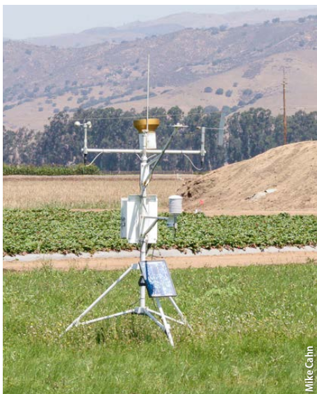
On-site CIMIS weather station provided accurate evapotranspiration data. Each N treatment was evaluated at two levels of irrigation — 110% and 160% of ET_c .
