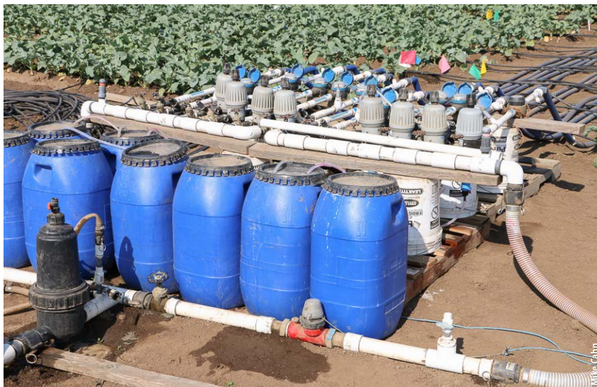
A manifold and injection system was used to simulate irrigation water with different NO 3 -N concentrations.
