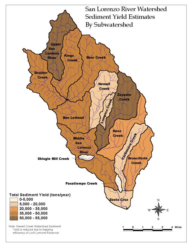
Figure 9 Sediment Yield (tons/yr) by Subwatershed
