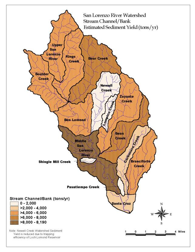
Figure 19 Stream Channel/Bank Estimated Sediment Yield
