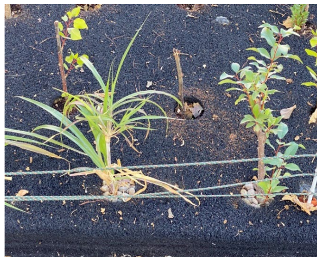
Figure 7.5 – The floating islands material is a synthetic, ultraviolet light resistant, mesh supporting plants.
