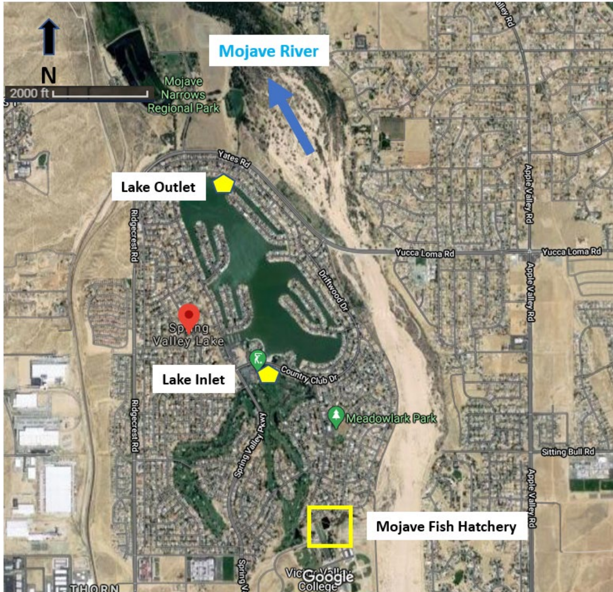
Figure 7.1 – Spring Valley Lake, west of the Mojave River is filled with groundwater pumped from 13 wells around the lake using about 2,200 acre-feet of water per year. In addition, the effluent from the CA DFW Mojave Fish Hatchery, containing elevated nutrients, irrigates the golf course before entering the southern end of the lake. At the northern end of the lake, an overflow weir discharges to the San Bernardino County Mojave Narrows Regional Park before returning to the Mojave River.
