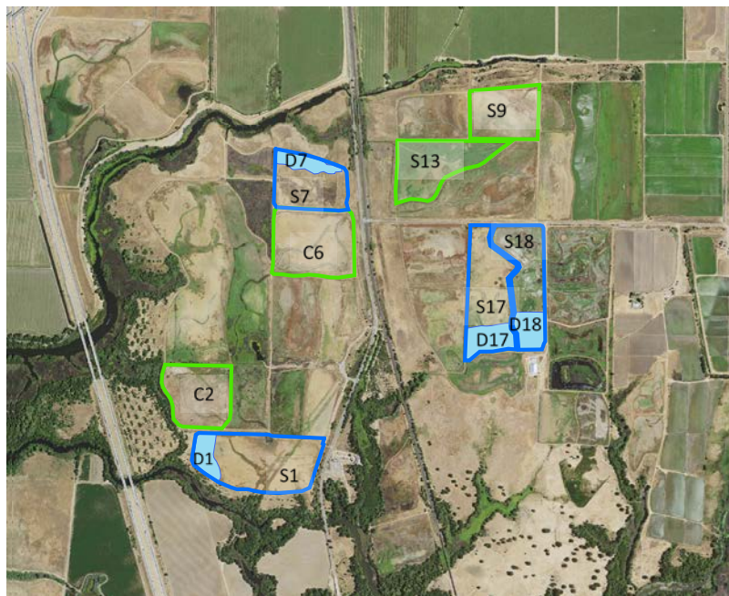
Figure 2. Four wetlands with deep-water treatment cells and an internal “check” levee were constructed (bordered by blue lines) and compared to 4 control wetlands (bordered by green lines) at the Cosumnes River Preserve demonstration area. The four control wetlands received traditional wetland management and will be monitored similarly to the treatment wetlands.
